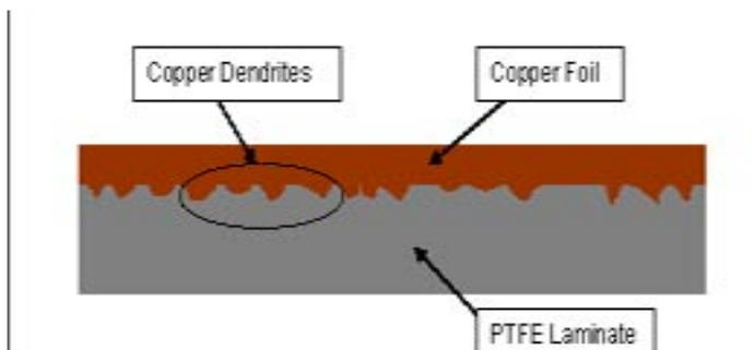
Figure 2 - Illustration of copper laminated to PTFE surface
